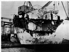
LORD NIAGRA'S STERN DAMAGE WAS REPAIRED AT SUN SHIP RECENTLY. The 377-ft. banana boat incurred the damage during a collision in the Delaware Bay. Fifteen tons of steel were used to repair the hull.
