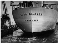
LORD NIAGRA'S STERN DAMAGE WAS REPAIRED AT SUN SHIP RECENTLY. The 377-ft. banana boat incurred the damage during a collision in the Delaware Bay. Fifteen tons of steel were used to repair the hull.
