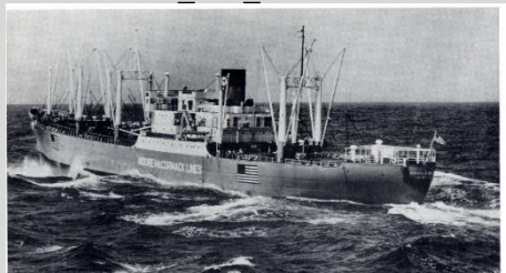
5.5: First cargo ship on the Maritime Commission Program to enter service. Here the M/S 'DONALD MCKAY' C-2 Cargo Vessel operated by Moore & McCormack is photographed in mid-ocean from its sister ship M/S 'MORMACDOVE'. Hull and propulsion equipment built at the Sun Yard. Photo ID: 500_175_04 8
