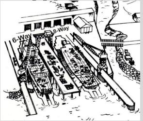
**5.1:** Drawing shows the conversion of the R-15 to R-25, 6 and 8 way 50-ton gantry cranes supporting 'Cab' structures. Drawings reflect the addition of approximately 30' elevation to the supporting structure enabling the cranes to support higher construction levels on the two new shipways. SSHS: 709\_315\_010\_02\_01
