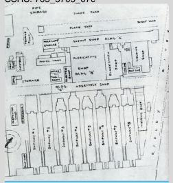
**3:1957/58 C.Y. Shop and Shipway Expansion** The shop removals were replaced with a relocated 1040' x 201'3" 'Layout, Fabrication & Assembly Shop' (A-1 high bay, A-2 low bay and A-3 low-low bay) that was previously located in No.4 Yard, disassembled and then reassembled in the C.Y. and became our 'Fabrication Shop'. This C.Y. expansion included the installation of two 880 ft. long shipways, No. 6 and No. 8, to support the construction of larger 50,000-ton and larger ships.
