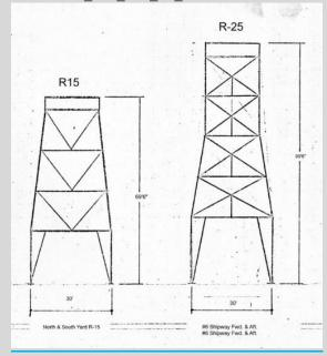
**5.2 Traveling (92') Bridge Gantry Cranes** Reconfigured R-15 Gantry structure to the R-25 'Traveling Bridge Gantry Cranes' installed between No.6 and No.8 Shipways was required to service ships on both shipways.
