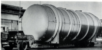
HEAVY'S TONNAGE IN THE NEWSPAPER came weeks ago when a big tank being hauled from Cleburne to Marlowe, Fla., backed up traffic. This is the tank and its 10th "Go" Ford for New York on midnight one night purposely to lower heavy-duty traffic as little as possible. See how close to ground trailer in that's what did happen. Going across an intersection which was a little high in center, trailer was left hanging with wheels in air, with all that weight on it what a job to get it off. But finally it was done.
