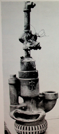
THIS IS a pump-grip. It is used to keep low spots (concretions, rollers, bridges) and the like free of water. That is it would be if someone hadn't broken it in big piece out of it. Now it won't be of any more use until broken spring is replaced. How did it happen? Who knows? Certainly men who did it isn't telling. Either it was dropped a long way or it was hit with a 100 lb. hammer. Pump cost $200 now. It will cost another $200 to put it in service again. This is one way by which our bill for repairing hand tools gets up to almost a quarter of a million dollars each year. Read page 2 in March magazine for figures for 1961.
