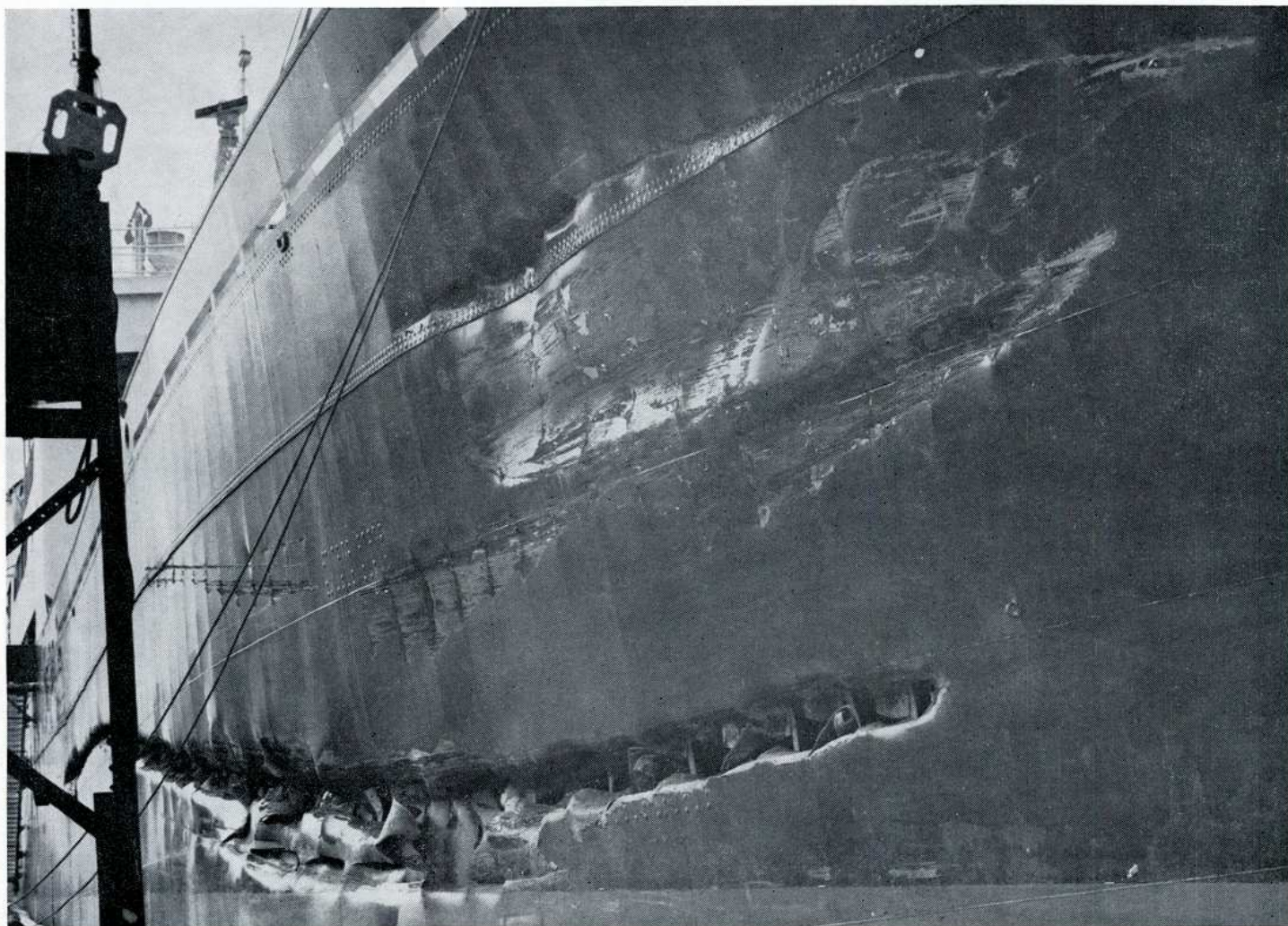
D'YUH DIG ME, KID? Whatever it was "Kid" was supposed to dig, it must have been real rib-ticklin'. In fact, Angela Fassio really split a gusset. Actually this rift was caused by passing acquaintance with anchor of a tanker in first snow storm of year last month. It was a nodding acquaintance, too, as can be seen by curve of gash. Italian cargo ship was repaired in less than two weeks.
