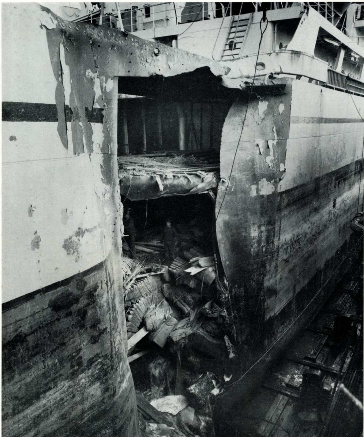
AFTER SEEING IT YOU FIND IT HARDER to believe a vessel could stay afloat with a gash in its side like that in S.S. Somerville. High and dry in dry dock in Our Yard, full damage to Norwegian freighter is apparent. Somerville and tanker, Sea Hawk, were in collision at mouth of Delaware Bay night of Feb. 13. Bow of tanker was smashed and she proceeded to Marcus Hook where she was emptied, inerted and then moved to dry dock (just a little too long for us).
