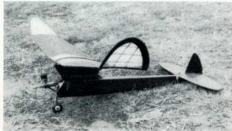
1.—Zeek Model Plane equipped with Bantam .19 engine, Austin Timer and D. E. Cutoff.
