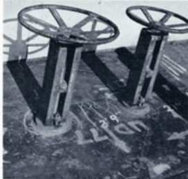
HAND WHEELS on the deck control the valves by shifting to the bottom of the cargo tanks. Deck stands are now fabricated in the shipyard some as bellmouths.
