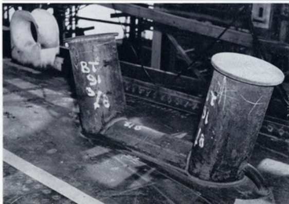
NEW BITT (discussed on opposite page) is shown welded to the deck of the first of three new 30,000 DWT tankships being built for Maritime for U. S. Navy use.
