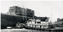
NEW TUGS are shown working S.S. ROCKY MOUNTAIN into place in the Basin following launching of the vessel in June.
