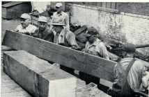
HEAVY TIMBERS are used in shipping large machinery and special gear units out of the plant on the east. It took five men from the Carpenter Shop to lift this block on the east.
