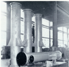
THE SHAPING MACHINERY (shown) will accommodate 100 lbs. cast iron 6" round length and 120" from the complete job of making pistons, castings, machining and hydraulic testing to 100 lbs. was produced at the Westfield Shop. The castings were made at United Machine Works, Albany, N. Y. Delivery was made in the summer of the late of one complete cast iron 100 lbs.
